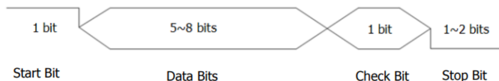
Figure 8.11 Schematic Diagram of UART Protocol
