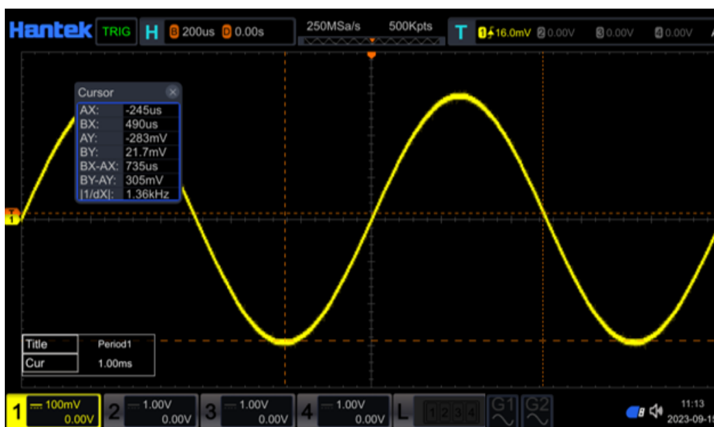
Figure 10.4 Track Measurement (after Horizontal Expansion)
