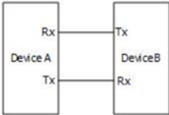
Figure 14.1 Schematic Diagram of UART Serial Bus
